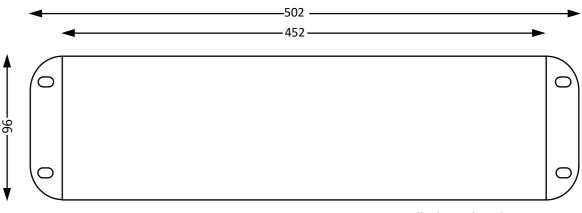
Fixing Holes M6 Product Height 60mm All Dimensions in mm Drawing not to Scale
