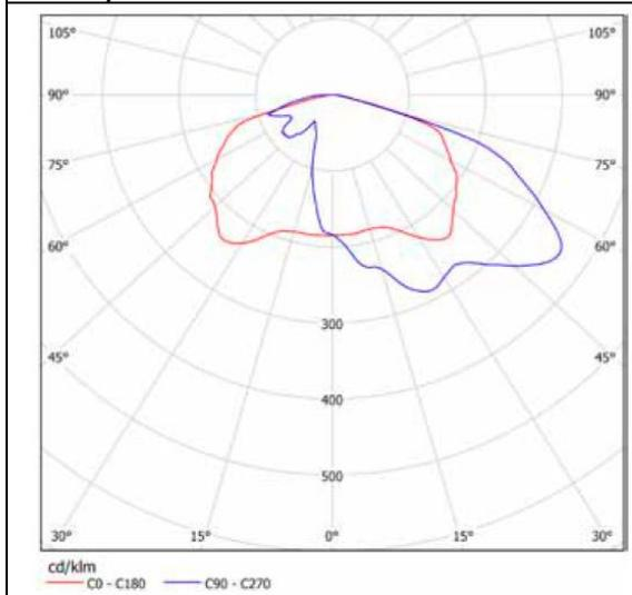
**SiliconCPV -DN** is a 2X2 array of asymmetric lenses suitable for area lighting. It has asymmetric forward tilted beam and wider light distribution than -FN.
