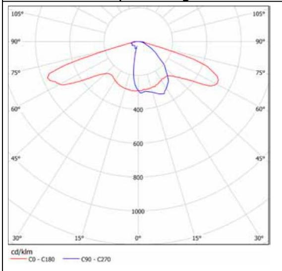
**SiliconCPV -DNW** is designed for roads where the pole height and the roadway width are similar.
