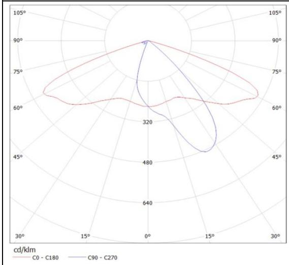
**SiliconCPV -ME** is the best of the class. Typical ME4a installations are possible with the ratio of pole distance and height up to 5.5. SCPV-ME is designed to fulfil ME-classes on a road whose width is equal to pole height or less.
