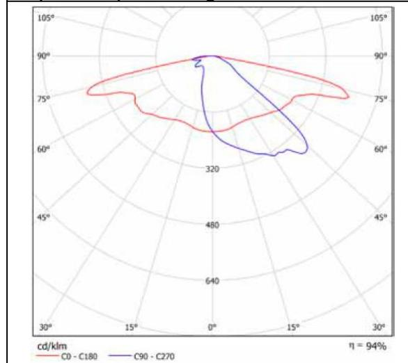
**SiliconCPV -DWC** is designed for roads with longer pole distances. It can be used in street lighting setups where the pole distance is six times the pole height.
